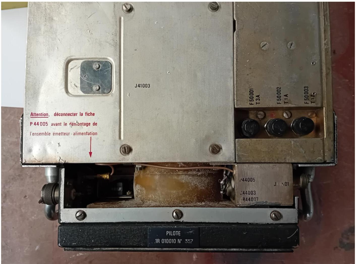
Top view, front part (left: driver & PA unit, right: Power Supply unit).
