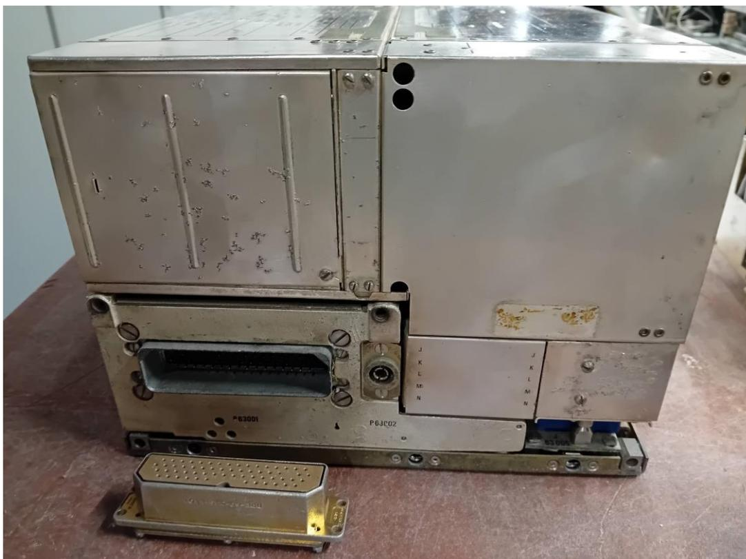
ER-104-A rear view (case removed) Note: connector ER-104 and 618T are identical. The ER-104-A and its control box fit straight in the 618T-2 mounting. The ER-104-A can't be combined with the 618T control box!!!
