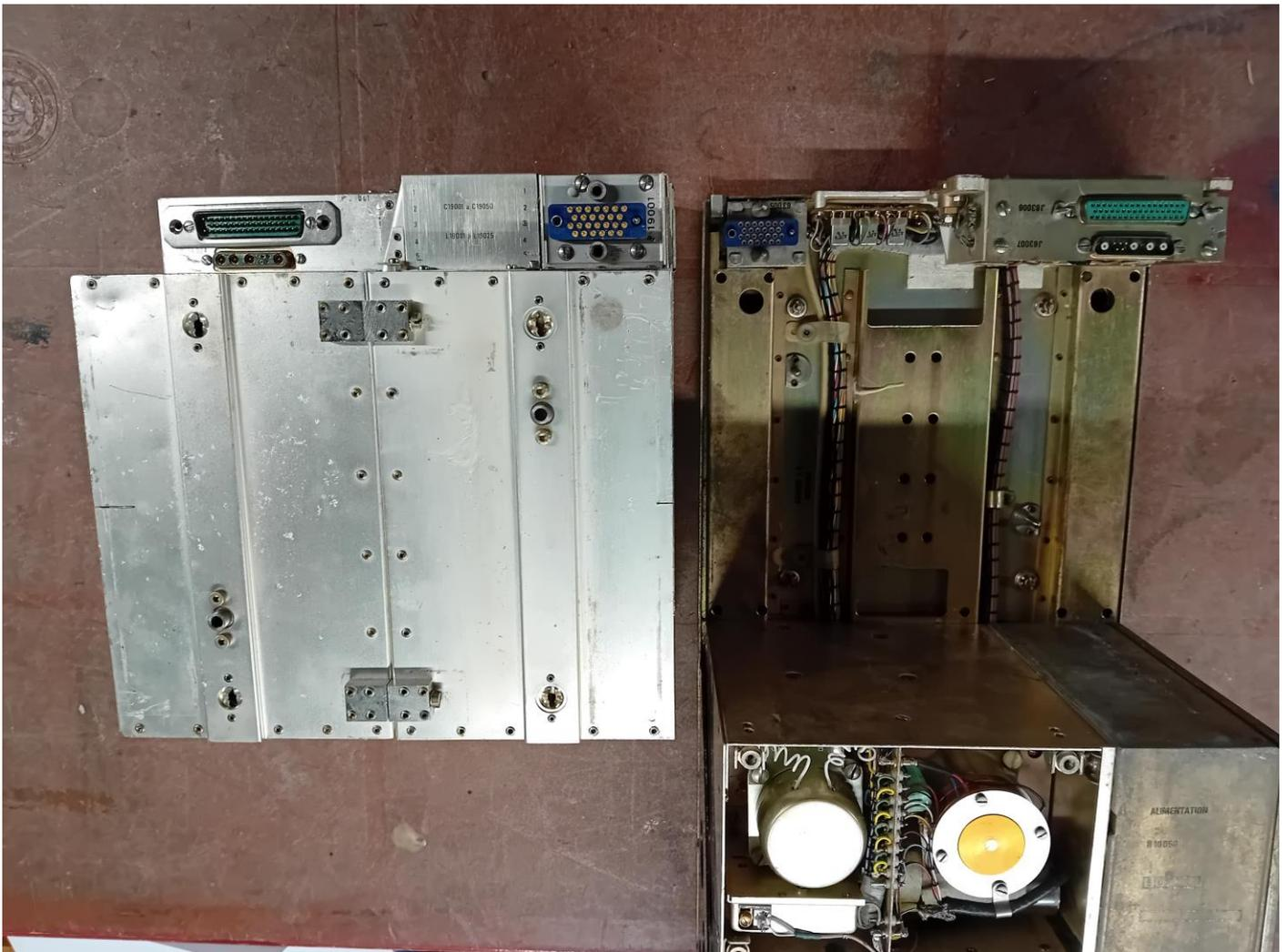
*Control- and Receiver unit removed from chassis.*
