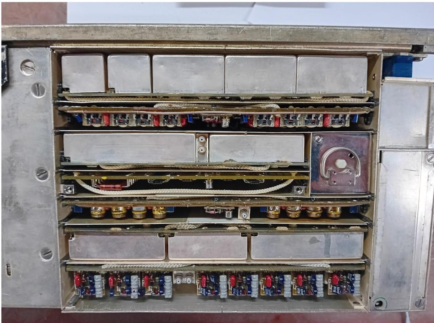
Modules of the **control unit**, left-back side of *trx*.
